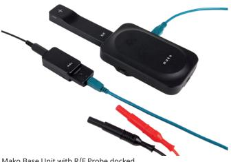
Mako Base Unit with R/F Probe docked, mAs Module connected and mAs cable.
