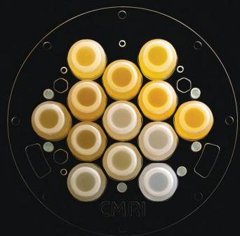
Contains the Liquid Crystal MR-Readable Thermometer, developed in collaboration with NIST. This ultimate, much-anticipated standardization thermometry is capable of standardizing between 15°C and 24°C. No ice bath necessary!
