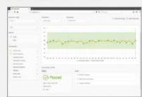
Each test parameter can be verified in a comprehensive trend analysis, allowing you to detect negative trends before your Linac will fail tests.
