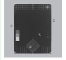
For diagnosis by using an X-ray film a suitable densitometer, (e.g. Unilight D / TR), for diagnosis at image display devices a luminance meter, class B according to DIN 5032-7, e.g. LXplus) is necessary.
