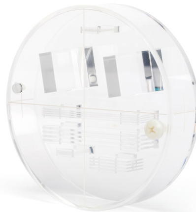
To4 - Spatial resolution (line pairs, MTF)
