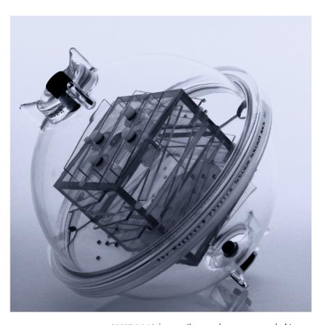
SPHERICAL MAGPHAN® (SMR100) is a urethane sphere composed of two hemispherical shells connected with a threaded ring. The shells together have an outer diameter of 21cm and an inner diameter of 20cm. The test cube assembly can be quickly removed without tools for greater imaging flexibility and easy access for cleaning and maintenance.
