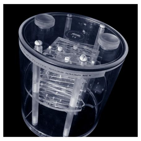
CYLINDRICAL MAGPHAN® (SMR170) is readily aligned in most conventional head and body coils. The acrylic cylinder has an outer diameter of 20cm and an inner diameter of 19cm.
