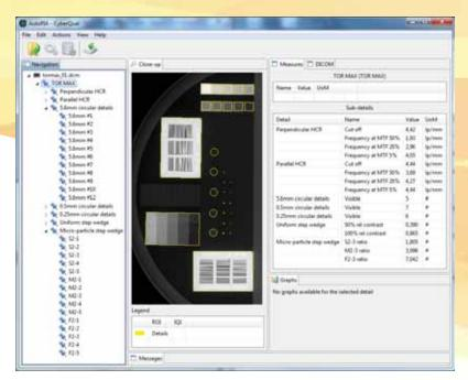
**AutoPIA** quickly provides objective, reliable and reproducible indices of image quality for routine quality control processes aimed at assessing the performance of X-ray systems.
