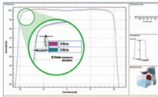
In-plane and cross-plane scanning consistency of Blue Phantom<sup>2</sup> with CC13 chamber
