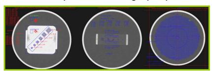
Connected to the QUALIMAGIQ platform, it takes only 2 mouse clicks and 10 seconds for the MOD-CTR module to analyze the DICOM images issued from the 1 to 4 sections of the phantoms supplied by scanner manufacturers (GE, PHILIPS, SIEMENS and TOSHIBA) and used for routine image quality controls of a CT-scanner.
