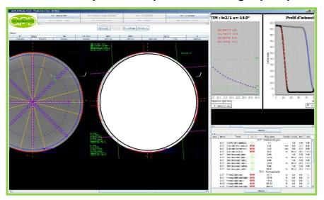
Connected to the QUALIMAGIQ platform, it takes the MOD-IRM-ES2 module only 2 mouse clicks and 10 seconds to analyze the DICOM images from the image quality control of a MRI installation.
