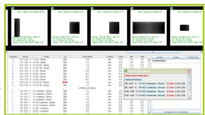
field sizes are given in relation to the X-ray collimator rotation axis. The software module also analyzes the concordances between the 3 types of fields.
