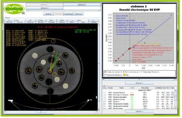
Connected to the QUALIMAGIQ platform, it takes only 2 mouse clicks and 2 seconds for the MOD-DE module to analyze every single DICOM image obtained with the CIRS 062 phantom, to construct the conversion curves of CT numbers – electronic densities and to control their constancy in relation to those registered in your TPS.
