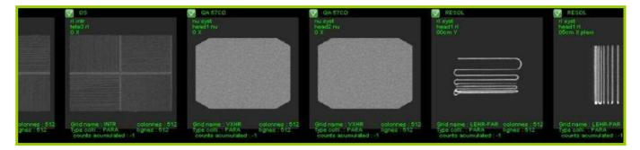
Connected to the QUALIMAGIQ platform, the MOD-PLANAR module takes only 2 mouse clicks and 10 seconds to analyze the DICOM images issued from a quality control of a gamma camera operating in planar mode.
