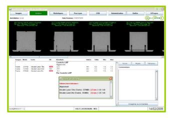
Automatic analysis of the control of the concordance between the external laser positioning system and the origin of CT-scanner dedicated for radiation therapy applications
