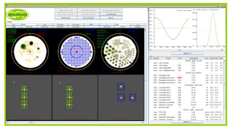
contrast, through analysis of the signals in the 6 cold spheres of the JASZCZAK phantom's section designed for this purpose: objective method based on a calibrated "software eye" which assigns a score in terms of number of visible targets.
