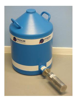
ITECH INSTRUMENTS N-type germanium coaxial detectors are useful down to ~3 keV, since they have a standard beryllium entrance window and a thin (0.3  $\mu$ m) P+ face. The NIGC extended range detectors are therefore the best choice for applications involving both X-ray and high-energy gamma-ray spectroscopy in the same sample.
