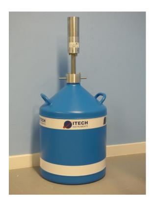
ITECH INSTRUMENTS P-type HPGe detectors have proven themselves worldwide over many years of unfailing service because they are manufactured in the past by PGT company. They exhibit excellent resolution and peak symmetry, with a useful energy range of 40 keV to 10 MeV. Efficiencies of 10 - 100% are available.
